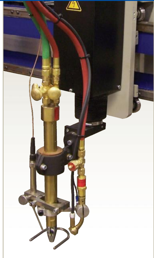
Shown with optional FT100 torch ignitor and Sensomat PAN automatic height sensing.
